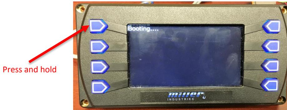
3. Use the 2<sup>nd</sup> and 3<sup>rd</sup> buttons on the right to toggle through the files until the correct file is displayed.
