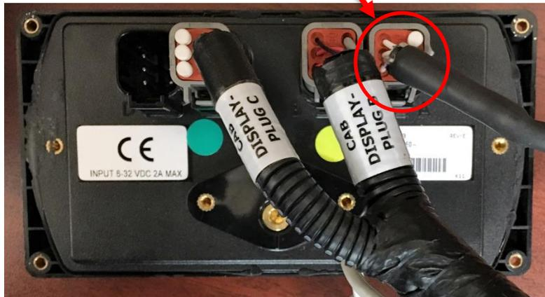
2. Press and hold the top left button on the display while turning on the trucks ignition switch. Release the button after 'Booting...' is displayed on the screen.
